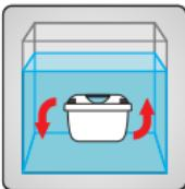
Place the cartridge into a container of cold tap water for 15 minutes. Then shake the filter once more to remove any air bubbles.
